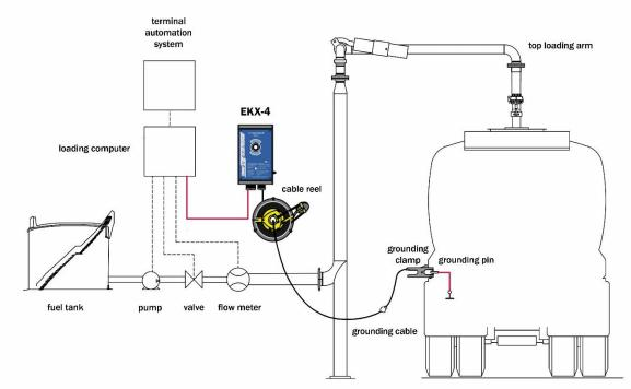
Figure 1: Monitored grounding with EKX-4 Grounding Control Device top loading vehicle
