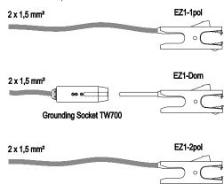
Figure 6: Grounding Clamp Configuration
