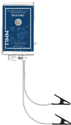
EZX-FIBC with integrated measuring electronics
